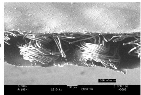
↑ **Figure** Scanning Electron Microscope (SEM) cross section of the cooling pad. Operational principle of cooling is a textile-based laminate of two waterproof, vapour-permeable polyester membranes  $\triangleright$ , which coat a hydrophilic fabric  $\blacksquare$ . By adding water (40 ml), evaporation leads to lowering of peripheral temperature.
